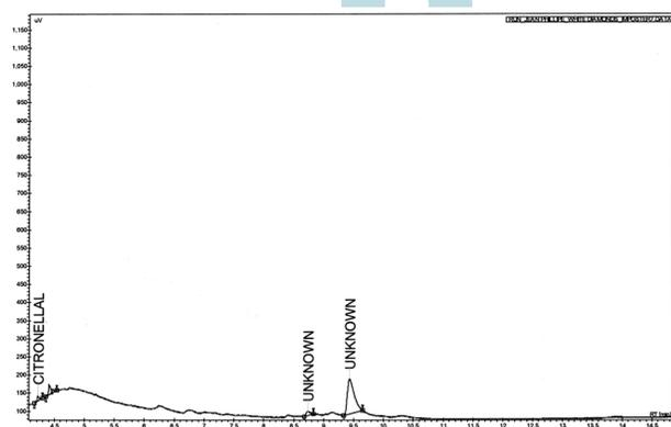
Figure 5. Imposter D Chromatogram. This fragrance had a refractive index of 1.3675 and 5 components integrating to 0.42% of the total composition.
