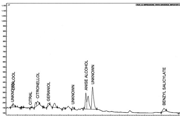
**Figure 4. Imposter C Chromatogram.** This fragrance had a refractive index of 1.3798 and 17 components integrating to 3.46% of the total composition.
