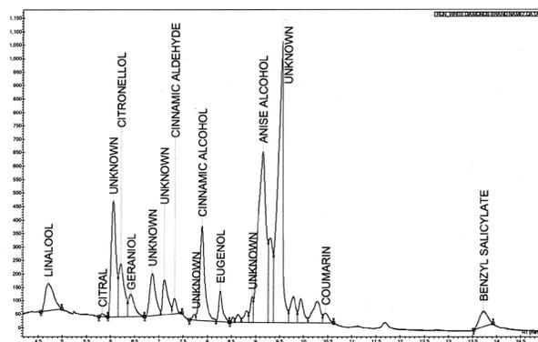
**Figure 1. Brand Name White Diamonds Chromatogram.** This fragrance had a refractive index of 1.3997 and 23 components integrating to a total of 19.81% of the total composition.
