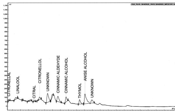
**Figure 2. Imposter A Chromatogram.** This fragrance had a refractive index of 1.3744 and 15 components integrating to 2.17% of the total composition.
