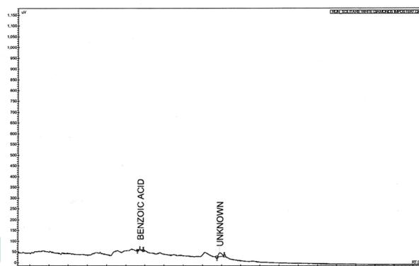
**Figure 3. Imposter B Chromatogram.** This fragrance had a refractive index of 1.3674 and 2 components integrating to 0.12% of the total composition.
