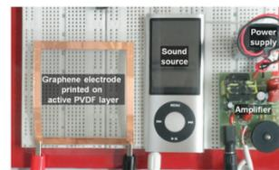
PVDF's flexible nature makes it a suitable material to form a diaphragm. Exploiting its piezoelectric effect, the material can contract and expand in response to a varying voltage (audio signal). When in
