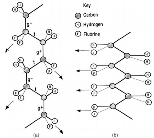
PVDF is a **ferroelectric** material with **pyroelectric** and **piezoelectric** properties. Piezoelectric materials react to mechanical stress by producing a potential difference. Pyroelectric materials also exhibit piezoelectric characters but also react to thermal changes by producing a potential difference. Ferroelectric materials, while also having piezoelectric and pyroelectric behaviours, can have their polarization direction altered under the influence of an electric field.
