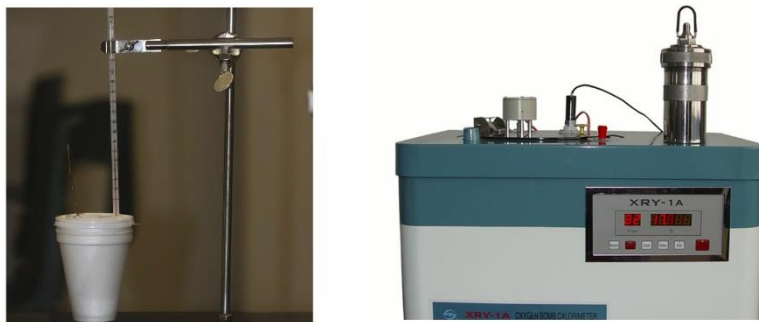
Figure 15: (Left panel) A coffee-cup calorimeter. (Right panel) A constant-volume calorimeter.
