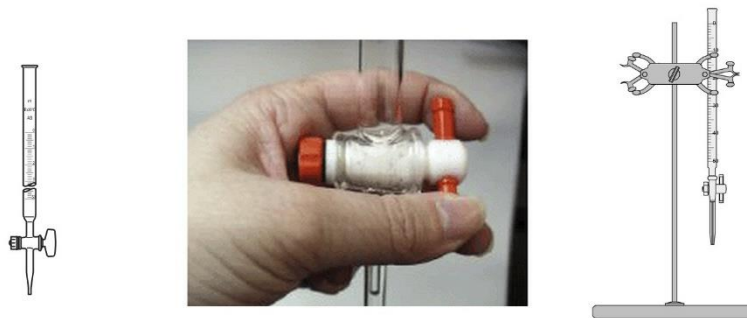
Figure 13: (Left panel) A buret employed in a titration. (Center panel) Illustration showing the correct way to control the buret valve. (Right panel) The titration set up
